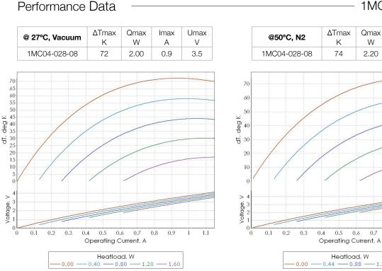
**Note**: Performance data is specified at optimal optimal conditions (TEC hot side is stabilized at ambient temperature). Any heatsink thermal resistance is not included into estimations. Use TECCad Software for estimations under different conditions.
